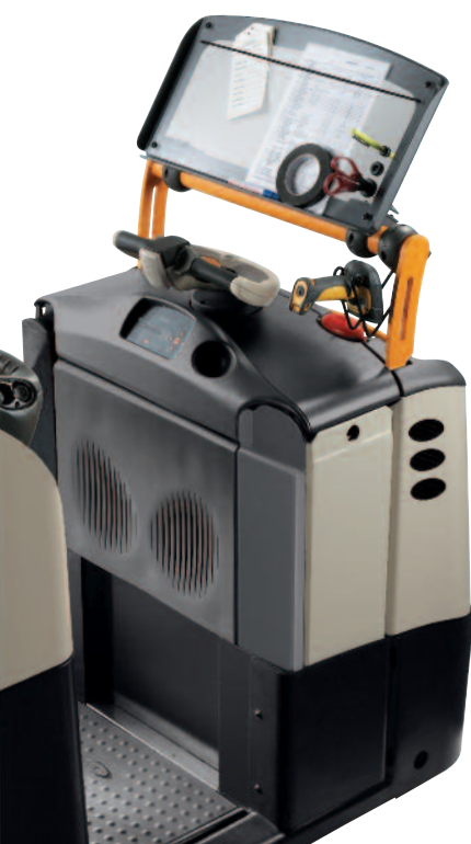
Front tube with large see-through clip pad and scan gun holder
