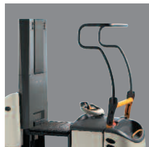
Lifting platform and picking guard (GPC 3040/3060)
